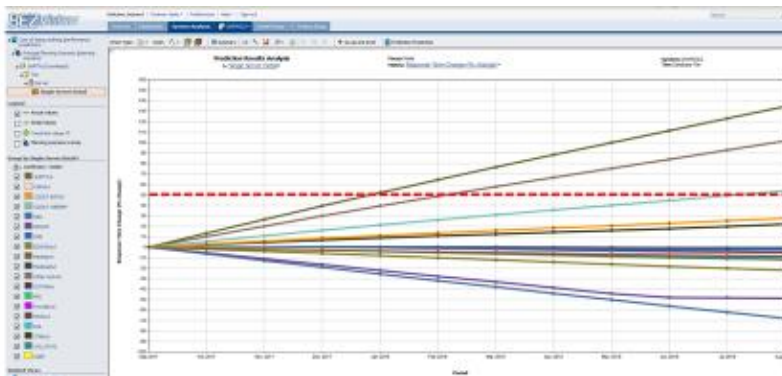
Figure 10. According to prediction results, Response time for three workloads (green, brown and blue) will not meet SLGs. Can changes in YARN Scheduler Queues required be determined to meet SLGs for all workloads?
