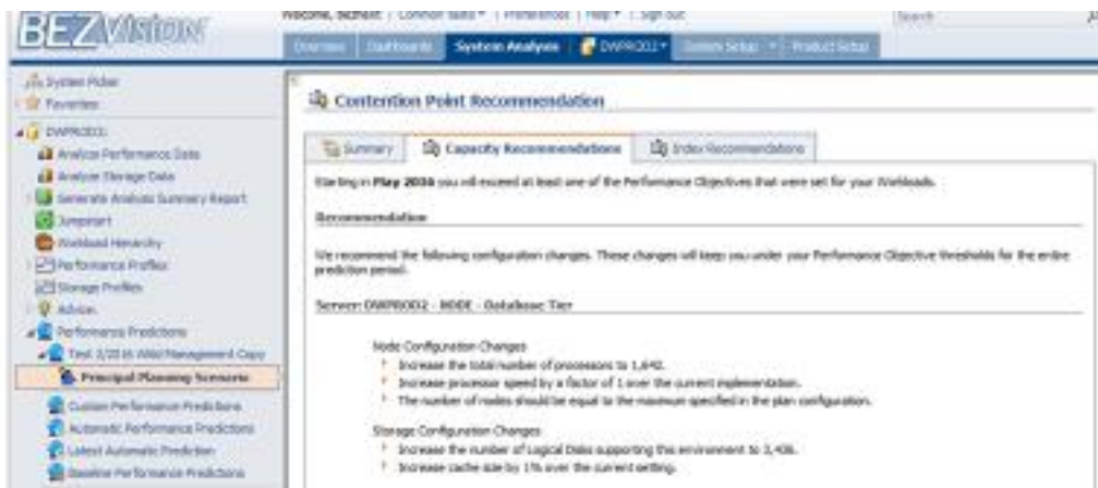
Figure 15. According to Capacity Planning Recommender increase from 1456 to 1642 CPUs and increase from 3432 to 3436 disks in a Cluster are required to meet SLGs for all workloads during next 12 months
